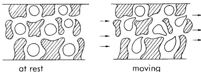
Fig. 9. In a porous oil bearing formation stagnant oil drops are spherical. In flow through narrow pores the drops must be deformed. This requires interfacial energy and an extra pressure drop, unless  $\gamma$  is very close to zero.
