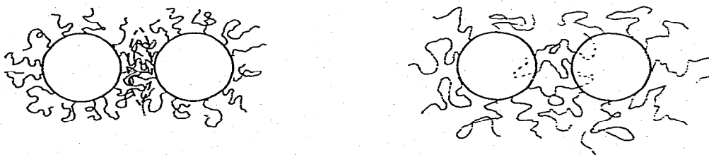
Figure 4 Illustrating the osmotic effect (left) and the volume restriction effect (right) in steric repulsion.
