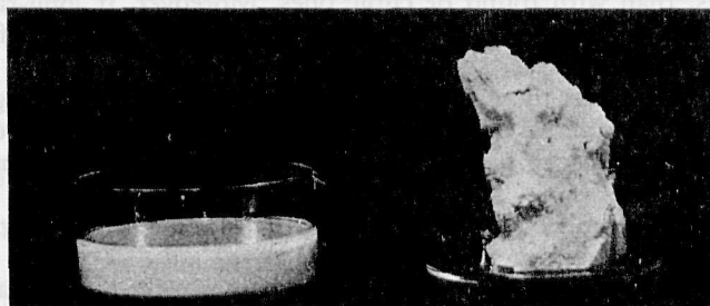
Fig. 8a. Starch (polar) in an apolar oil (xylene). Left: Completely dry. Fluid. Right: Starch contains 12% water. Solid.
